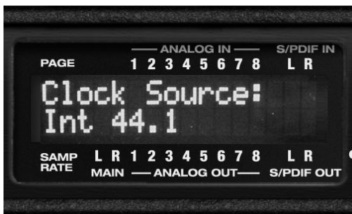
Figure 6-2: In setup mode, the LCD displays a setup parameter in the top row of the LCD and the current setting in the bottom row.
