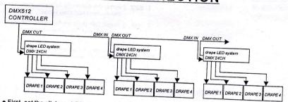
First, set the all drape LED system as DMX 24CH mode, then connect DMX512KT with each system in parallel.
