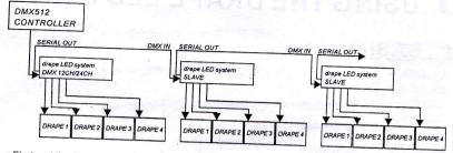
First, set the first drape LED system as DMX12CH or 24CH mode, other systems as slave mode.
