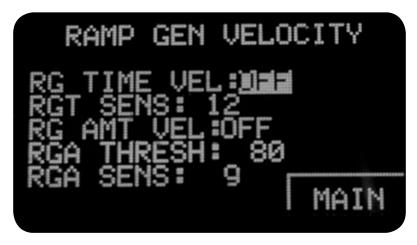
When in the RGV menu, press shift + RG VEL to turn all RGV response ON. Use this button combination again to turn all RGV response OFF. When RGV response is ON, then RGV will be highlighted in the lower left corner of the display in the MAIN menu.
