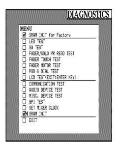
6) The Cursor should be pointing to exit, press **ENTER**. The DM is set back to Factory Default.
