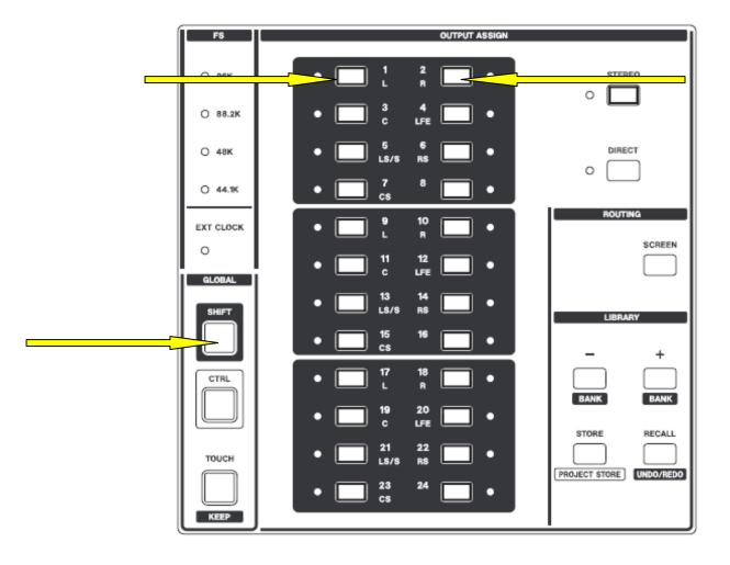
3) While holding down these buttons, power up the **Dm 3200 or 4800**. At the top of the LCD screen, you should see **Diagnostics Mode** on startup and the screen will switch to the main **Diagnostic** Page.
