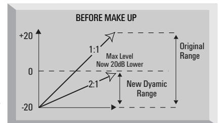
For example, in the diagram the compressor reduces the signal by 20 dB, which reduces the dynamic range of the input and in so doing makes the signal quieter.
