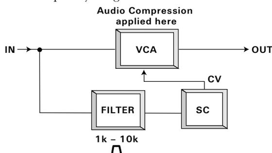
The exciter is the opposite of the de-esser - it amplifies the selected area of the frequency spectrum. It is good for resurrecting an old recording, or for restoring the dynamic range of an instrument, so putting life back into it and letting it sit higher in the mix.
