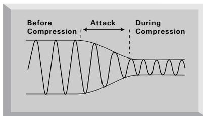
Transient response is less affected, so maintaining the presence of each note.
