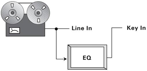
Now, you can use the key input to control the compression of the original signal. The original signal is compressed as if the dominant instrument had been attenuated.
