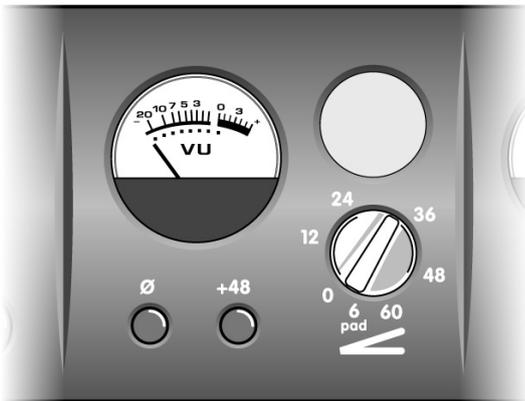
The gain control is switched, and has 12 positions. The first position gives -6 dB gain, in other words it attenuates (reduces the volume of) the signal, and is for use with microphones that have very high output levels. Each subsequent position increases the gain by 6 dB, up to a maximum of 60 dB.
