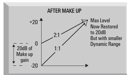
Using the make-up gain restores the volume of the compressed signal.
