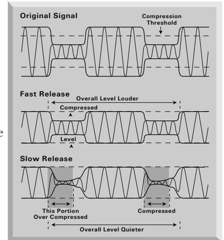
You do not have to set a permanent release time for the whole input signal; instead, you can use the Auto button. Auto reacts to the dynamic range of the input, so the higher the signal is above the threshold, the longer the release. This means that fast signals that aren't compressed hard have a fast release time, while longer signals release more slowly, which makes the compression in context with the signal.
