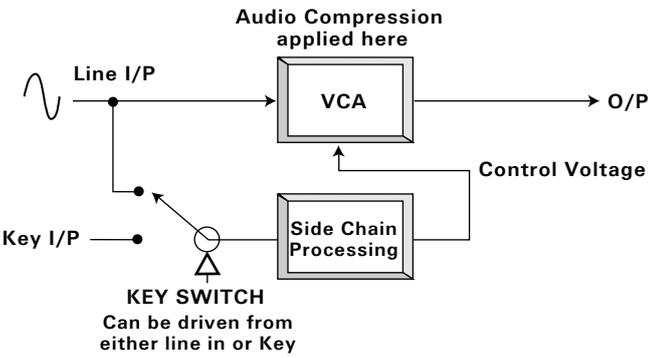
key input. Note that the key input signal is not output from the unit, it is the original input that is compressed, but compression is applied as if the key input signal were being compressed.
