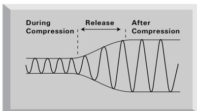
Loudness is determined by the maintenance of high mean levels: compression increases the proportion of high-level signal content, and as the diagram shows, the faster the unit releases, the more low-level signal is brought to a higher level. Therefore, the faster the release rate, the higher the perceived loudness of the recording.
