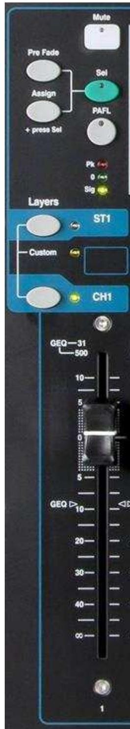
**Mute key** – Press to turn off the channel audio signal. This affects the send to all mixes including LR, effects and stage monitors. The Mute key lights red when the channel is muted. It flashes when it is muted by a Mute Group master.
