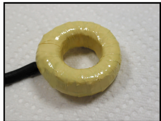
Fig. 1b The heart of the VintageWindings EQ-1A Complete Filter Unit. This tapped Toroid coil is also available separately.
