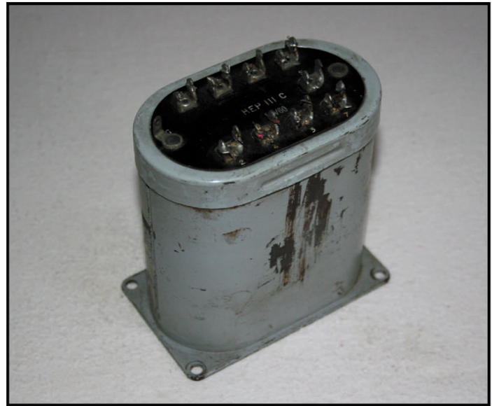
Fig. 4 The Western Electric 111C toroidal line transformer. Super overkill in this application but these make for a very nice sounding vintage EQ, a very heavy EQ that is.
