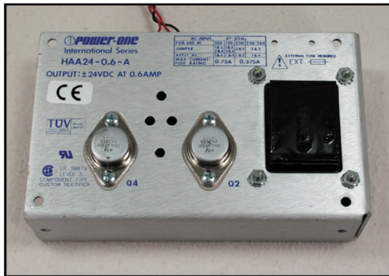
Fig. 6 Power One HAA24-0.6-A power supply. It's fairly bulletproof and has good regulation. The voltages are also adjustable for rail balance.
