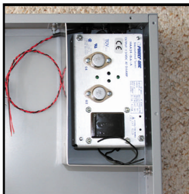
Fig. 9 Power One HAA24-0.6-A power supply. It's fairly bulletproof and has good regulation. The voltages are also adjustable for rail balance. The photo to the left shows the simple hand bent shield that surrounds the power supply. I have used these power supplies without the shield with no problems. The shield is used here to keep the AC to the power switch away from the audio circuit and is overkill. See Figs 18ab Page 15.
