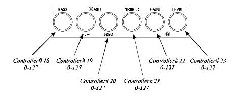
Note: Program changes can not occur when operating in Continuous Controller mode.
