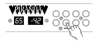
② Use the UP and DOWN buttons to change the current HUSH threshold value. To set the threshold properly, listen to the noise floor with the threshold set at its lowest setting (-70) while not playing. Increase the threshold value until the noise is no longer audible. (Use caution, as setting this value too high will cause the downward expander to attenuate the output too quickly and not allow the signal to decay as long as it should.)
