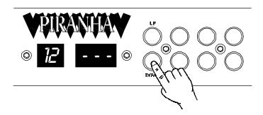
② Use the front panel knobs to adjust the parameters until the desired sound is achieved. (The store button will blink after any preset parameter has been changed from its stored value.)
