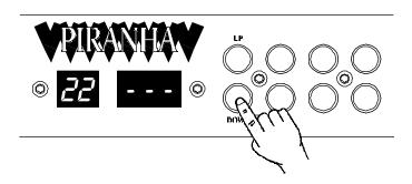
**2** Without making any parameter changes, press the STORE button three times to store the current preset as the Power-up preset.
