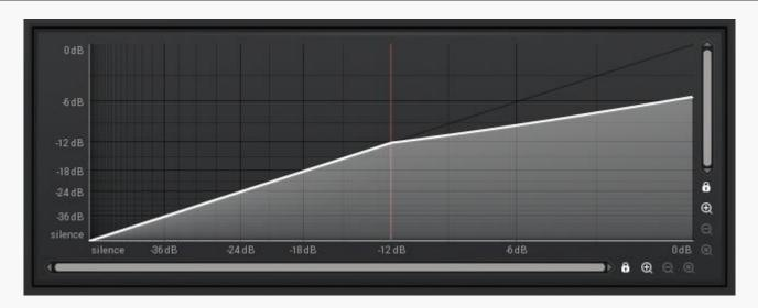
Signal graph defines the compression envelope. X axis represents input level, Y contains the output level. You can edit it if you enable **Custom shape**.
