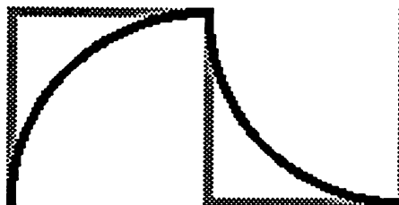
Square Wave before and after Lag Processor
