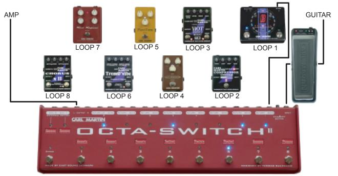
Connect a tuner to i.e. loop 1 send, and nothing in the loop return, select i.e. program 8 with only loop 1 engaged, this way you mute the system while getting signal to your tuner, without the signal passing through the tuner.
