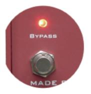
The Octa-Switch has nine switches, the eight are presets and the ninth is a true bypass switch, which bypass the unit for clean sound. Please note if the buffer is engaged it will also be engaged in the bypass mode, which we recommend as on large stages when running long connected cables, there is a definite drop in the high end of your guitar sound, the buffer prevent that.
