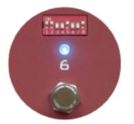
Then by turning on or off the numbered switches in each of eight DIP Bank switches, you determine which effects you wish to use simultaneously in each Bank. There is a blue LED for every effects loop used and for each Bank (so once you are programmed, when you step on Bank 6 you will see the lights of all the effects you have assigned to Bank 6 and the Bank 6 LED).
