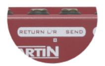
Loop 8 offer a mono send and a stereo return on a stereo jack plug, with left at the jack tip and right at the jack ring. The Octaswitch has stereo outputs, and a stereo return on Loop 8 (this is a stereo jack with tip-left and ring-right). Since stereo effects like choruses are placed at the end of your effects-chain, we would typically insert them in Loop 8.
