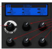
• Turn Knobs I thru 5 to adjust the selected effect's parameters
