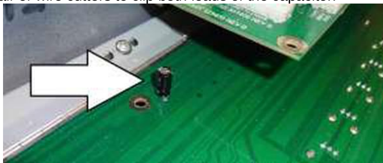
Figure 1 – C7 on Left Front Panel PCB
