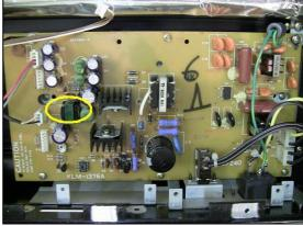
Now on to the modification. You'll work in the area marked in yellow above. First remove the two wire jumpers as indicated on the pictures below:
