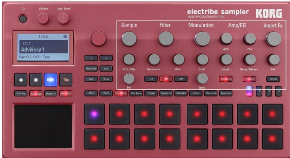
The “electribe sampler” lets you load any sample from an SD card and use it for producing beats. There are 499 user sample memories in which you can store original waveforms that you've created using waveform editing software or sampled sources provided by developers. Of course you can also connect a record player or instrument to the audio in jack and sample from it.
