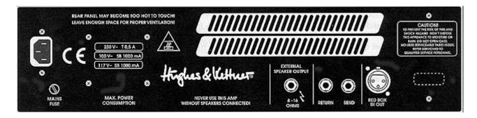
MAINS IN: Connect the included Euro-norm mains cord to this socket. Ensure the amp's voltage rating matches your local AC voltage rating before you plug the cord into the wall socket.
