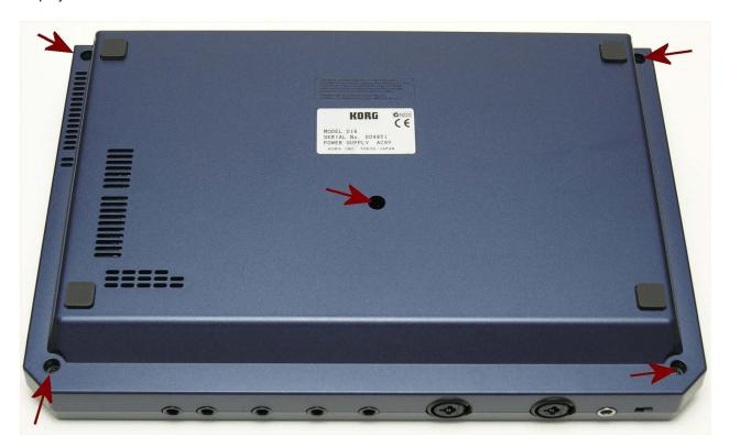
The case is held together with 5 cross-head screws, arrowed. Unscrew them and keep them safe along with the other small parts already removed.
