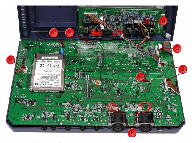
Lift the bottom of the case carefully. There are two wiring looms that connect the small circuit board in the lower half of the case to the main mother-board.
