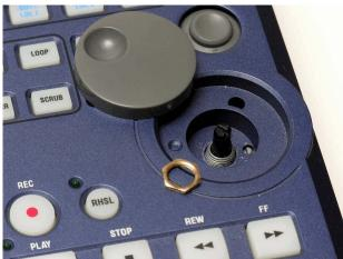
The Value Dial knob is removed in the same manner as the trim knobs. Once it is removed you will see the retaining nut for the Value dial encoder, this should be removed with the 11mm ( $^{7}/_{16}$ ") socket-spanner or by careful use of point-nosed pliers.
