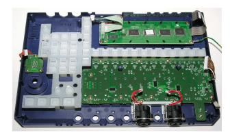
You may need to manouevre the motherboard slightly, to ensure that the LEDs and buttons line up with the top panel.
