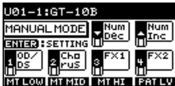
Manual mode is enabled when this screen is displayed.
