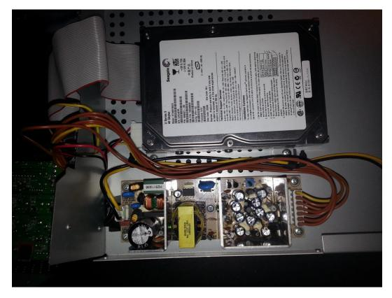
The hard drive is mounted on two rails which are attached to the bottom assembly using 4 Phillips head screws.
