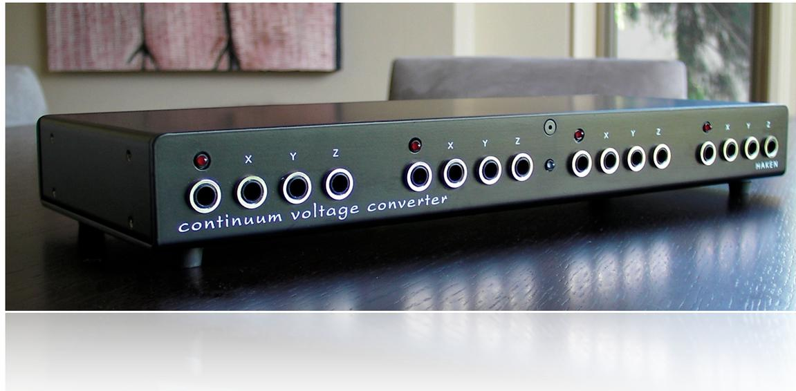
Haken Audio's Continuum Voltage Converter is designed for use with analog control-voltage synthesizers. The CVC converts the polyphonic X (pitch), Y (front-back), and Z (pressure) outputs of the Continuum Fingerboard into control voltages and gates. Alternatively, user-defined preprocessed control voltages can be defined with the EganMatrix.
