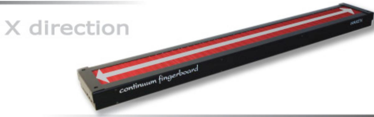
*The X direction of the Continuum Fingerboard is generally mapped to pitch.*
