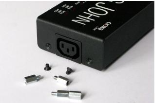
Then attach the pairs of stand-offs to the power supply and tighten using the bracket as a wrench. Plug in the adapter and fasten the bracket on top of it using the included two screws.
