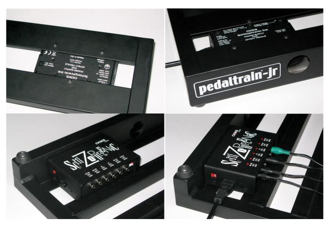
On the next page you see how two link range power supplies are mounted underneath a Pedaltrain board and powered with just one mains power cord. The LINK adapter is placed between the two units and passes the AC mains from the first unit to the second one. The AC Rider link on the right has a courtesy AC mains outlet free to be used as you please ex. with the universal mains adapter – the MAda, described later in this document.
