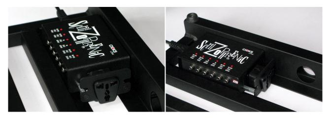
When the link range power supply is mounted underneath the Pedaltrain board as described earlier in this document, the adapter allows powering of two different devices like ex. a plug-on adapter – one plugged in from the top and one placed underneath the board as shown on following two pictures.
