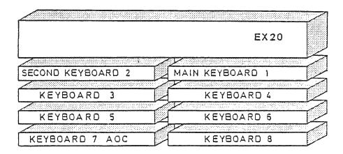
The following chart shows the corresponding names between the MK 1 and EX 20 keyboards:
