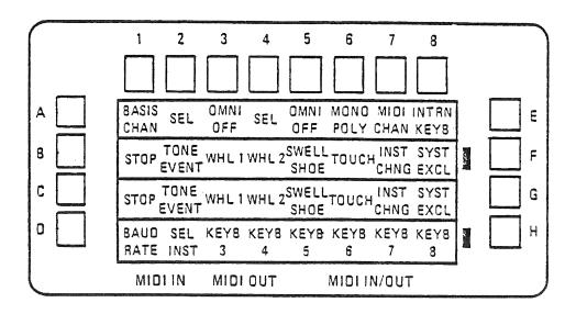
The EX 20 automatically selects the MIDI Level of the Function Control Matrix after being turned on.
