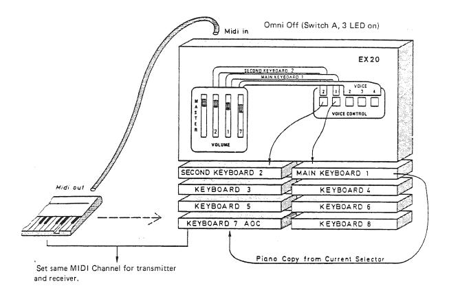
The DMS Instrument "Piano" is now copied into "AOC 7" and can be accessed through MIDI. Make sure that the MIDI transmitter and receiver are using the same MIDI channel.
