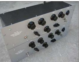
This is about as close as you can get to a real vintage Pultec EQP-1a. Built from the original Pulse Technologies <u>Pultec schematic</u> with the <u>layout</u> designed around modern replacement parts (filter caps and trannys); and utilizing best practices regarding lead dress and component placement. Parts cost is around \$1100 USD.
