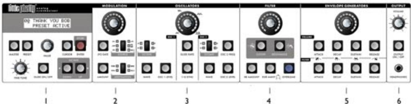
1. The LCD display and User Interface - provides controls to access presets and other software functions. The Fine Tune control is located here, along with switches for Glide On/Off and Octave transpose.
