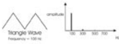
Like the square wave, the triangle wave only contains odd harmonics, but the levels of the harmonics in a triangle wave are much less. The triangle wave has a soft, slightly buzzy sound that is suitable for high-pitched leads (like a flute) or adding a beefy sub-bass to bass sounds.
