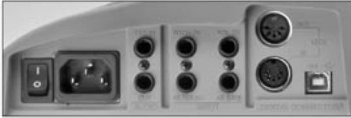
The Side Panel provides all of the input and output connections. In addition to Audio Input/Output jacks, there are CV and Gate inputs, connections for MIDI, and the power connector and power switch.
