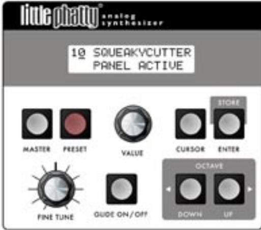
Preset sounds are selected using the **VALUE** knob. As the **VALUE** knob is advanced, the next preset appears in the display and is immediately available to be auditioned (you do not need to 'activate' the preset to hear it). Pressing **VALUE** and turning the knob will advance by increments of ten.
