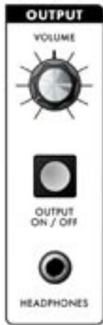
The Little Phatty has a single monophonic audio output. The level of the audio output is adjusted by the Volume Control. An On/Off switch allows you to turn off the output signal while keeping the Headphone signal active.
