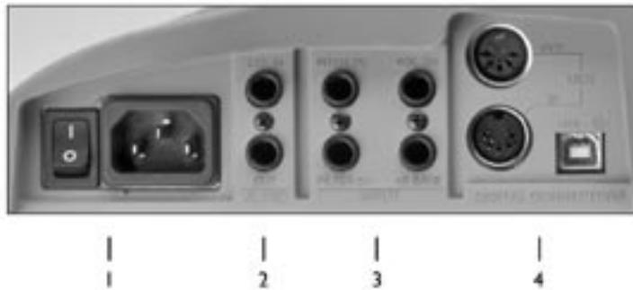
1. Power Socket and Switch – provides power to the LP. Power is ON when the switch is in the up position.
