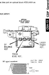
Clear RF signal waveform means that the shape " $\Diamond$ " can be clearly distinguished at the center of the waveform.
